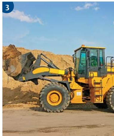
This is the best piece of plant for excavating foundations. We use it to dig out earth and
